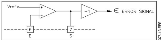
Output and inverting input are accessible thus giving high flexibility in use. The non-inverting input is not accessible and is internally connected to  $V_{REF}$  (or  $0.9V_{REF}$  in burst mode - see paragraph II.6)
