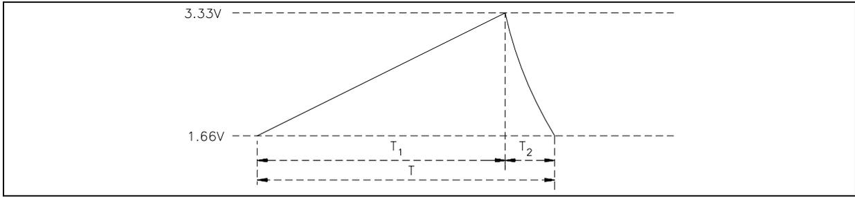
$C_O$  capacitor is charged with a constant current. The current is fixed by  $R_O$  which is supplied by voltage  $V_{REF}$ .
