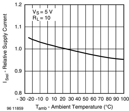
Figure 5. Rel. Supply Current vs. Ambient Temperature
