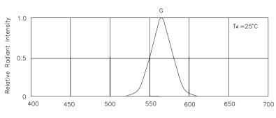
wavelength  $\lambda$  (nm) RELATIVE INTENSITY Vs. WAVELENGTH
