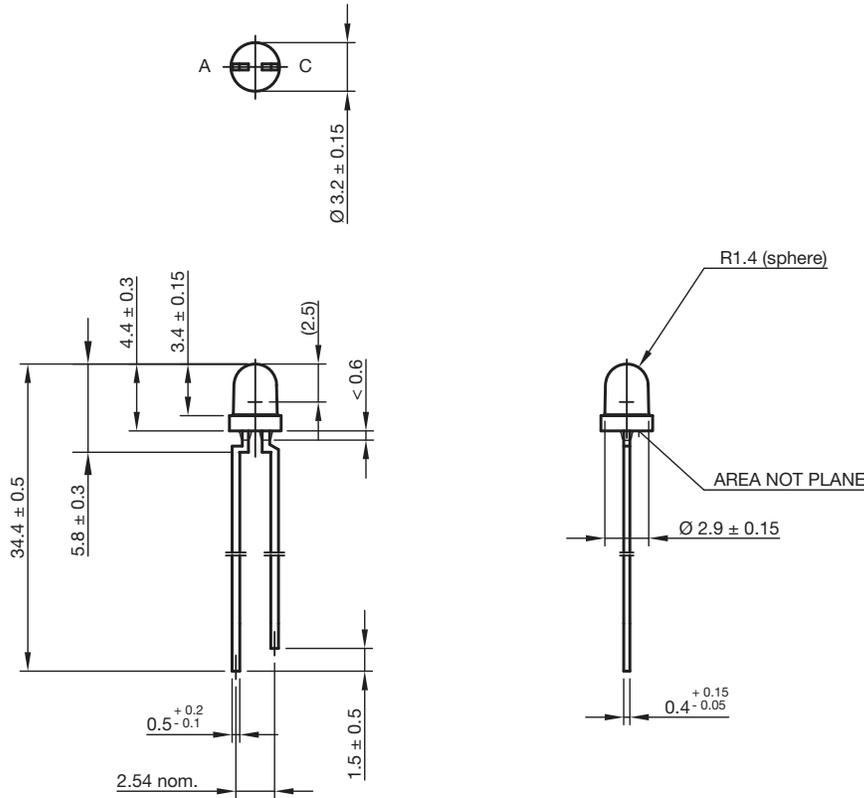
technical drawings according to DIN specifications
