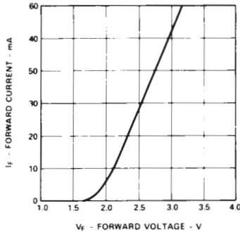
Figure 7. Forward current vs. forward voltage characteristics
