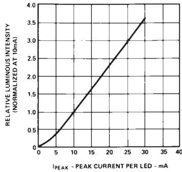
Figure 13. Relative luminous intensity vs. DC forward current
