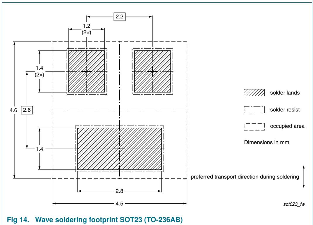
Fig 14. Wave soldering footprint SOT23 (TO-236AB)
