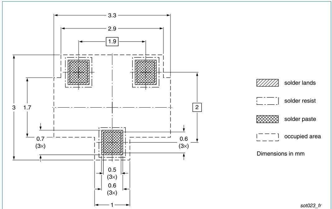
Fig 13. Reflow soldering footprint SOT23 (TO-236AB)
