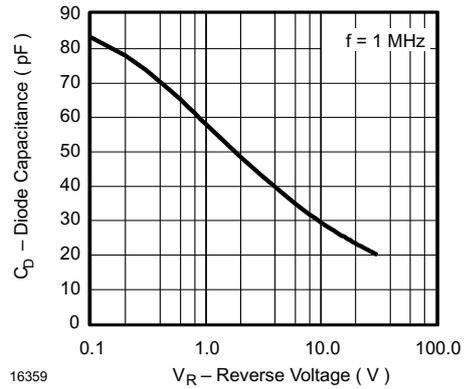
Figure 6. Diode Capacitance vs. Reverse Voltage
