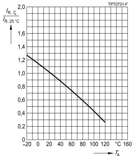
**Characteristics (typical) for  $T_{ref} = 120\text{ }^{\circ}\text{C}$**
