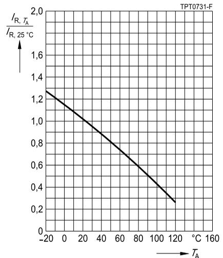
Characteristics (typical) for  $T_{ref} = 130\text{ }^{\circ}\text{C}$
