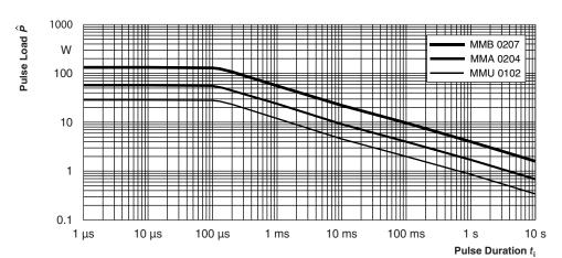
Maximum pulse load, continuous pulse; applicable if  $\bar{P} \leq P$  ( $\mathfrak{d}_{amb}$ ) and  $\hat{U} \leq \hat{U}_{max}$ ; for permissible resistance change  $\pm$  (0.5 % R + 0.01  $\Omega$ )
