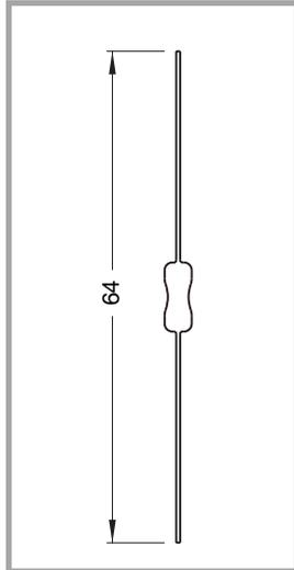
**Fig. 8: Axial preformed**
