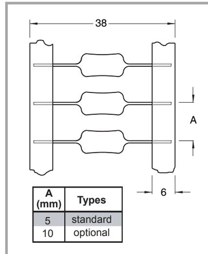
**Fig. 5: Radial Taping**
