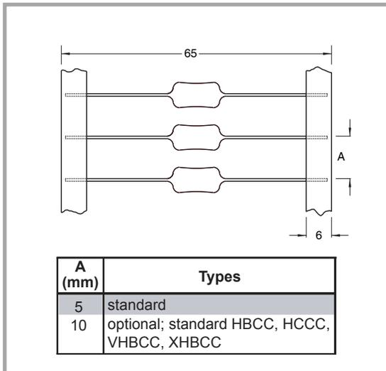
**Fig. 4: Axial Narrow Taping (38mm)**
