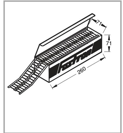
**Fig. 3: Axial Standard Taping (65mm)**
