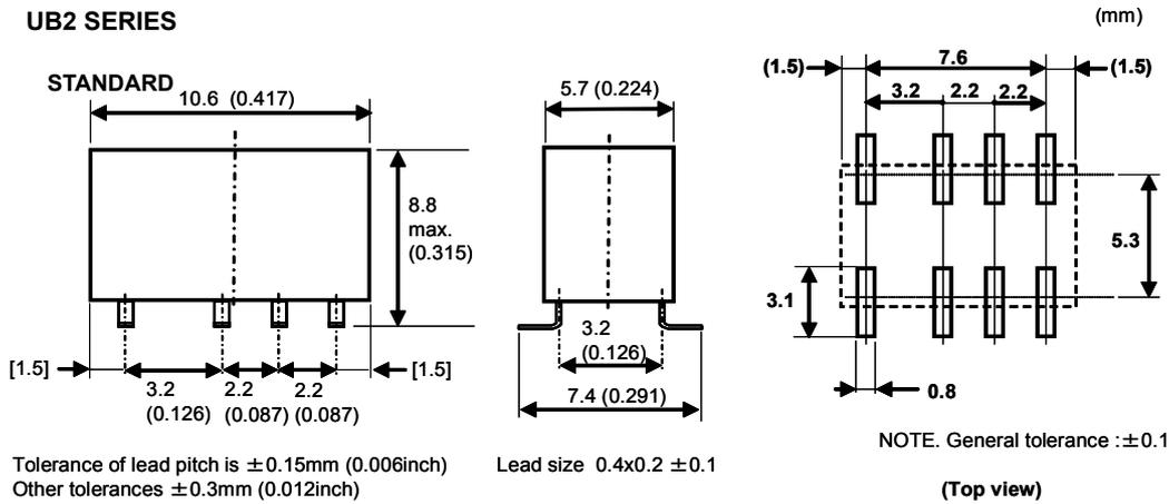
Tolerance of lead pitch is  $\pm 0.15\text{mm}$  (0.006inch)
