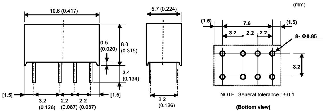
Tolerance of lead pitch is  $\pm 0.15\text{mm}$  (0.006inch)
