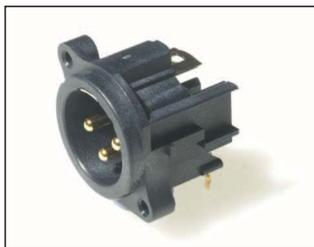
**XNACM5 / PC90 3 Pin horizontal PCB mounting male XLR for self-tap screw fixing. Gold plated Brass contacts. Vertical PCB mounting also available, part XNACM5 / PCS. Optional EMI / RFI Screen.**
