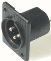
XACM / PCS 3 Pin vertical PCB mounting Male XLR with non counter sunk mounting holes for self-tap screw fixing. ACM PCS has counter sunk mounting holes for M3 screw fixing. Nickel Silver plated Brass contacts.
