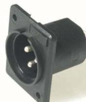
XACMR / PC 3 Pin horizontal lateral right PCB mounting Male XLR with non counter sunk mounting holes for self-tap screw fixing. Nickel Silver plated Brass contacts.
