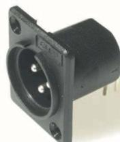
ACM / PC 3 Pin horizontal PCB mounting Male XLR with counter sunk mounting holes for M3 screw fixing. XACM / PC has non counter sunk mounting holes for self-tap screw fixing. Nickel Silver plated Brass contacts.
