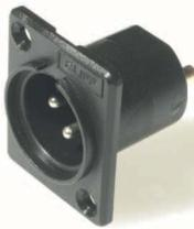
ACM 3 Pin chassis mounting Male XLR with counter sunk mounting holes for M3 screw fixing. XACM has non counter sunk mounting holes for self-tap screw fixing. Nickel Silver plated Brass contacts.
