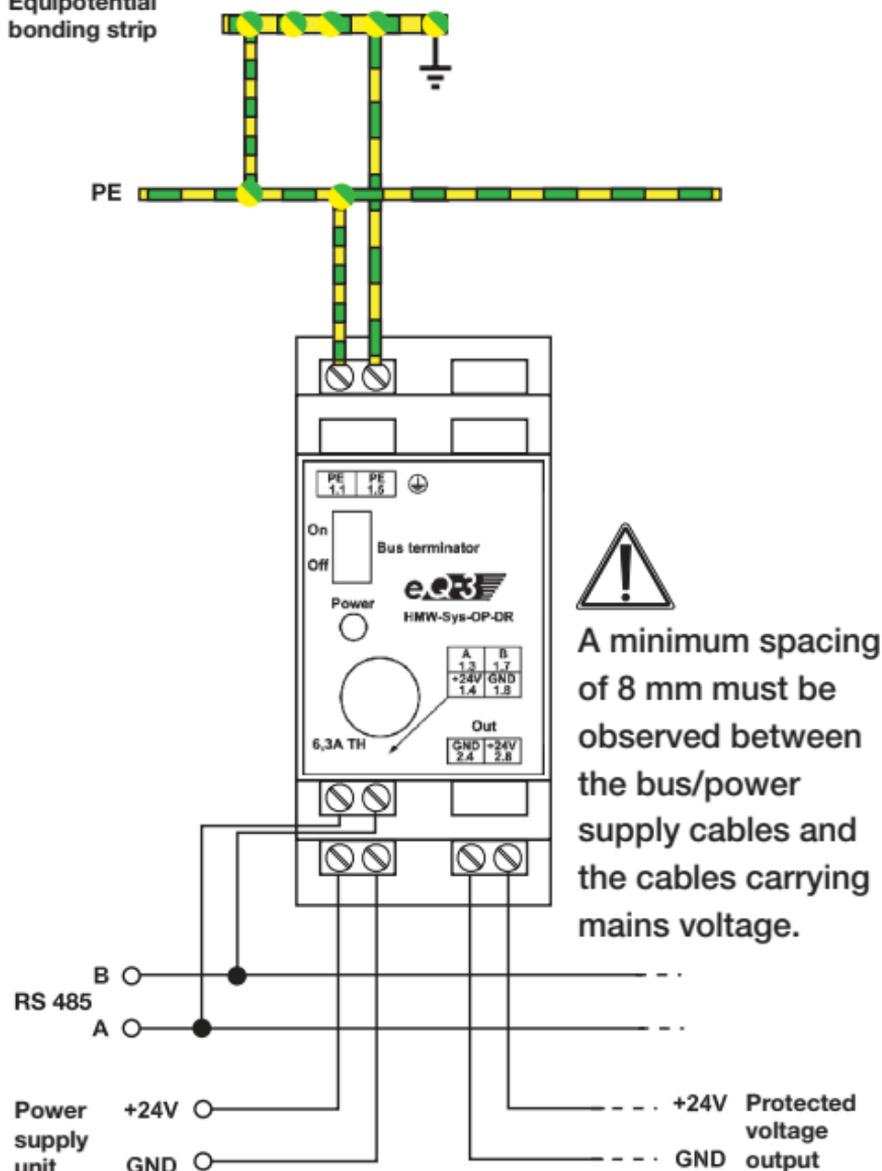
First of all, wire the connection to the PEN (protective conductor) busbar in the distribution board and to the equipotential bonding strip that is connected to the foundation earth. When doing so, observe the following notes:
