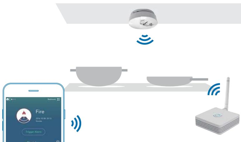
Receive the alarm if smoke or heat detected
