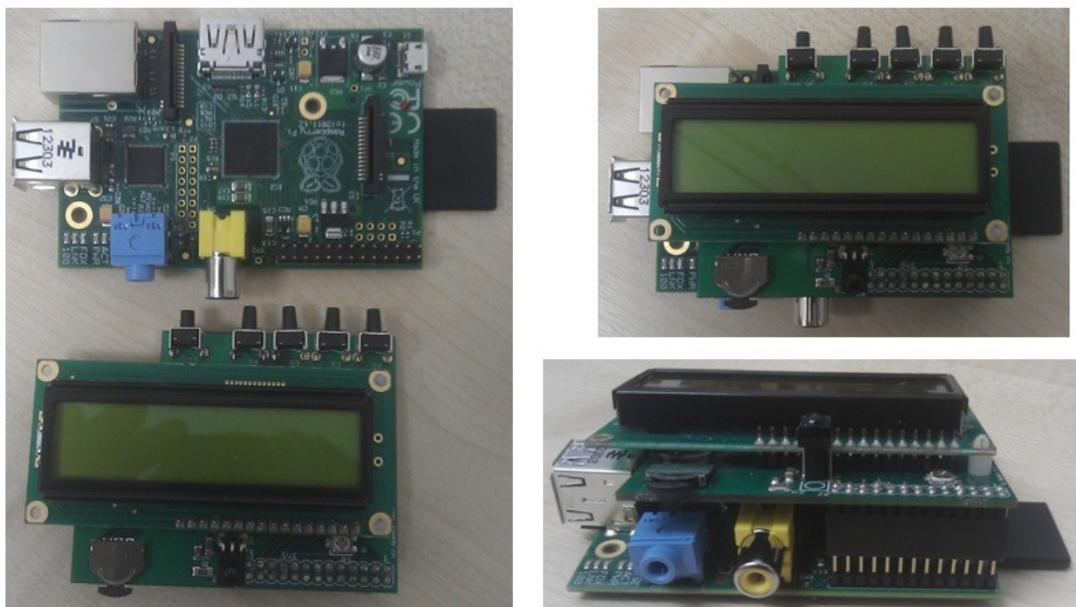
*Figure 1: Raspberry Pi & PiFace Control & Display Setup*
