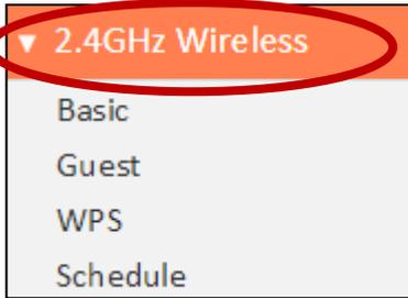
The “2.4GHz Wireless” & “5GHz Wireless” menu allows you to configure SSID and security settings for your Wi-Fi network along with a guest Wi-Fi network. WPS, access control and scheduling functions can also be managed from here.
