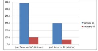
Thanks to the Gigabit Ethernet available on the ODROID-C1, the network performance of C1 is an impressive four to six times faster than Raspberry Pi.
