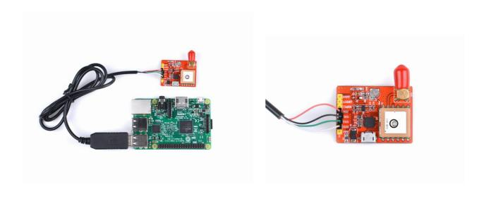
**USB Style:**Just use a microUSB cable connect Raspberry Pi USB port with GPS module and power on Raspberry Pi.
