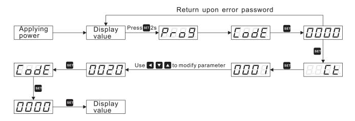
Example 2: The factory default parameter is AC 5A(CT=1); If the current transformer is 200A/5A, should modify the CT multiplying power as 40(200/5)
